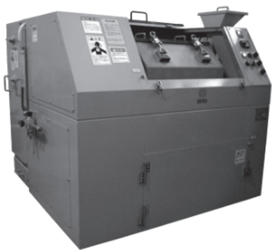
Fig. 10 Dry type rotating barrel machine
