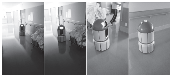
Fig. 4 A robot that automatically avoids dolly
