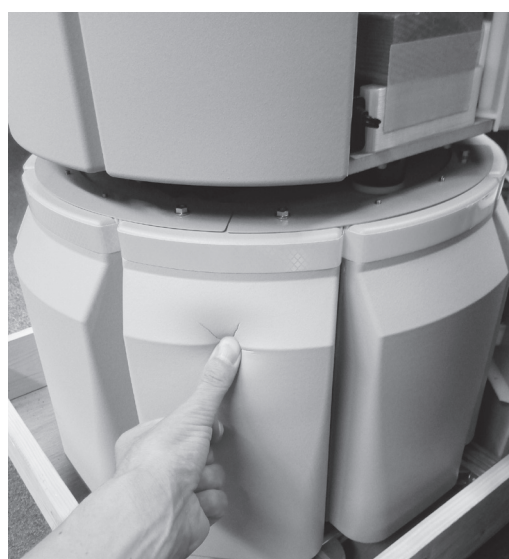
Fig. 6 Flexible exterior with contact detection function
