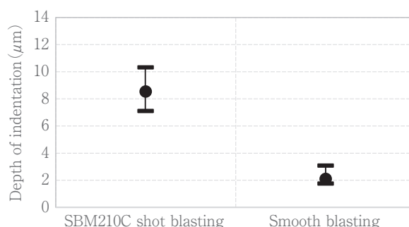
Fig. 13 Depth of indentation measurement result.
